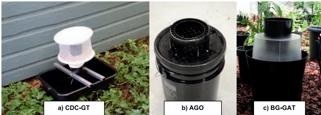
Fig. 1. Mosquito gravid traps used in current comparison study: (a) Centers for Disease Control and Prevention (CDC) Gravid Trap (CDC-GT) used as standard, (b) Autocidal Gravid Ovitrap (AGO), and (c) Biogents Gravid Aedes Trap (BG-GAT).
